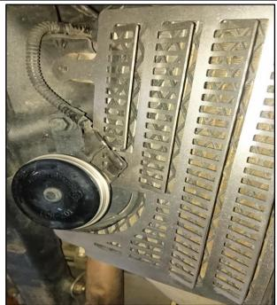
9. Fasten the LHS Radiator Guard using the below Fastening Kit and OE Hex Screws.
