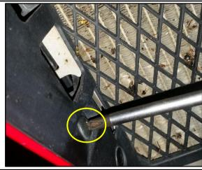
2. Remove the 2 x Hex Head Screws on the RHS Radiator as indicated.
