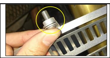
4. Using the below Fastening Kit fasten the RHS Radiator Guard as indicated.
