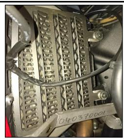
6. Remove the OE HEX Screws and OE Screw on the LHS Radiator as indicated.
