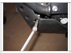
4. Push the longer bolt through the little hole on the LH of the bash plate with a #5 Allen key – make sure it goes al the way through the bracket and engine mounting point
