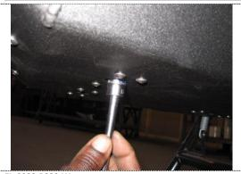
3. Hand tighten the M8 Nylock nuts using a #13 socket as illustrated
