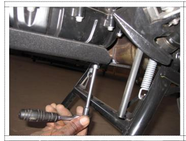
8. Firmly tighten the bottom of the bash plate to the rubbers using a #13 socket as illustrated
