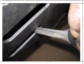
6. Carefully push it through one of the RH fins on the front of the bash plate positioning it over the bolt to tighten as illustrated
