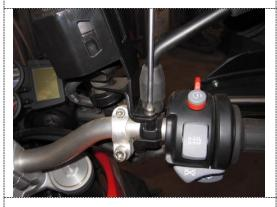
2. Position reservoir protector over both holes, re-insert bolts and tighten as per photo (you may need an extra hand to hold and balance the mirror and bracket while tightening)
