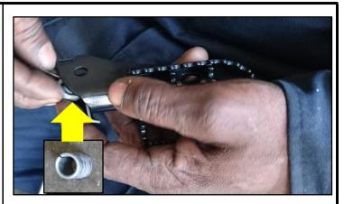
4. Place the Wide Foot Peg into the Foot Peg Mounts as indicated and replace the Pin removed in Step 1.
