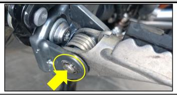
2. Once the OE Foot Peg is removed the Foot Peg and Spring can be discarded.
