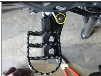
5. Replace the Circlip removed in Step 1.
