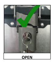
2. Press the lever inside the latch upwards and lift as indicated.
