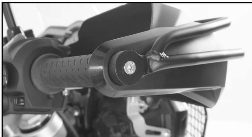
Fastening of the handle protection bar left and right top:
