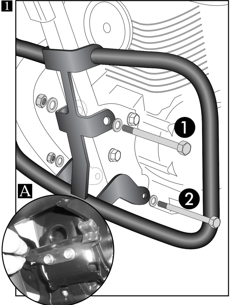
Unhook the clutch cable and change the position as visible in the picture.
