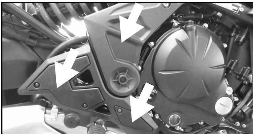
Remove the three marked original screws and the original spacers. Screws and spacers are obsolete.
