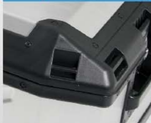
Case and top case have several integrated slots for belt fastening
