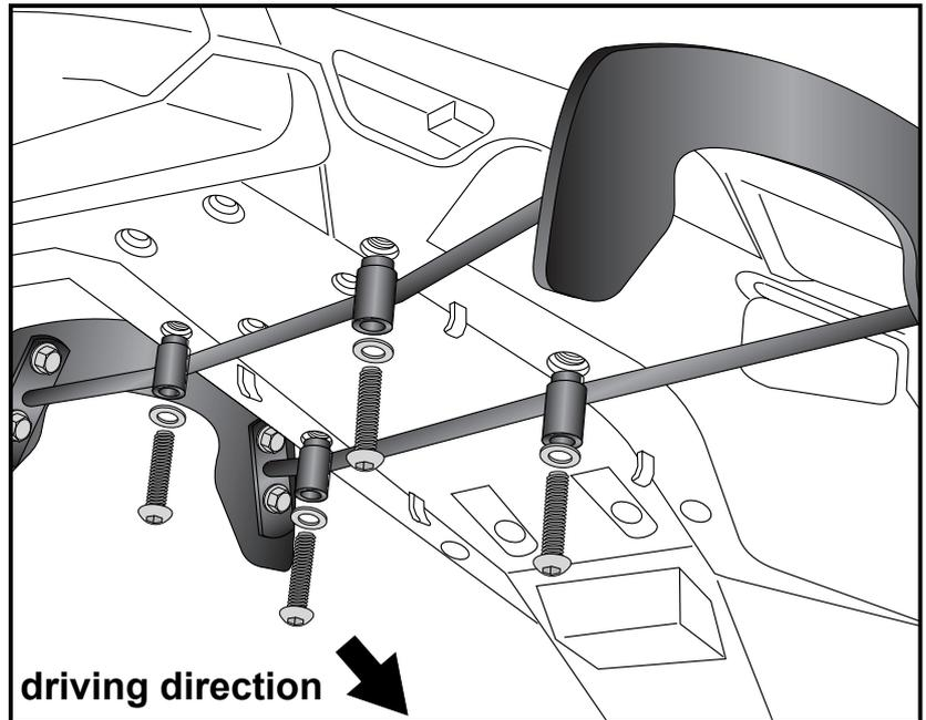
Control all screw connections after the assembling for tightness!
