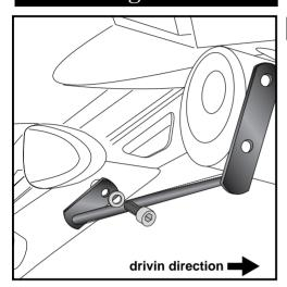
Fastening of the C-Bow adapters left + right rear: at the fixing point of the adapter, mounted in step 1 with allen screw M8x20 and washers Ø8,4.
