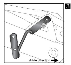
Fastening of the C-Bow adapters left + right front: at the fixing point of the exhaust with the original screws.
