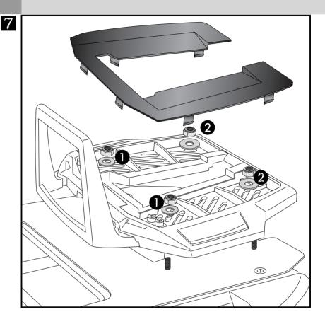
Control all screw connections after the assembling for tightness! Please notice our enclosed service information.
