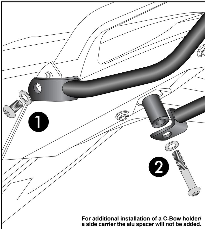
For additional installation of a C-Bow holder/
