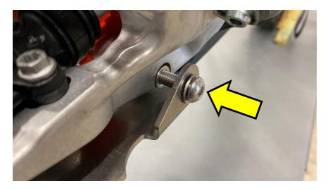
(5mm HEX) Snug the 8mm bolt, nesting the RMCG into the machined part of the foot bracket.
