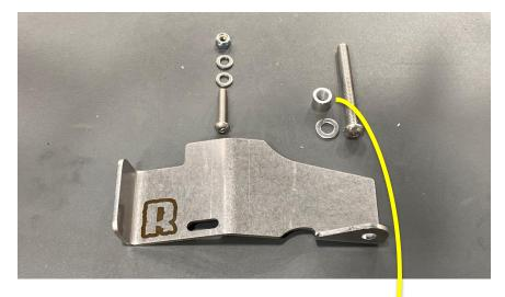
Load the provided aluminum spacer I to the foot bracket cavity.
