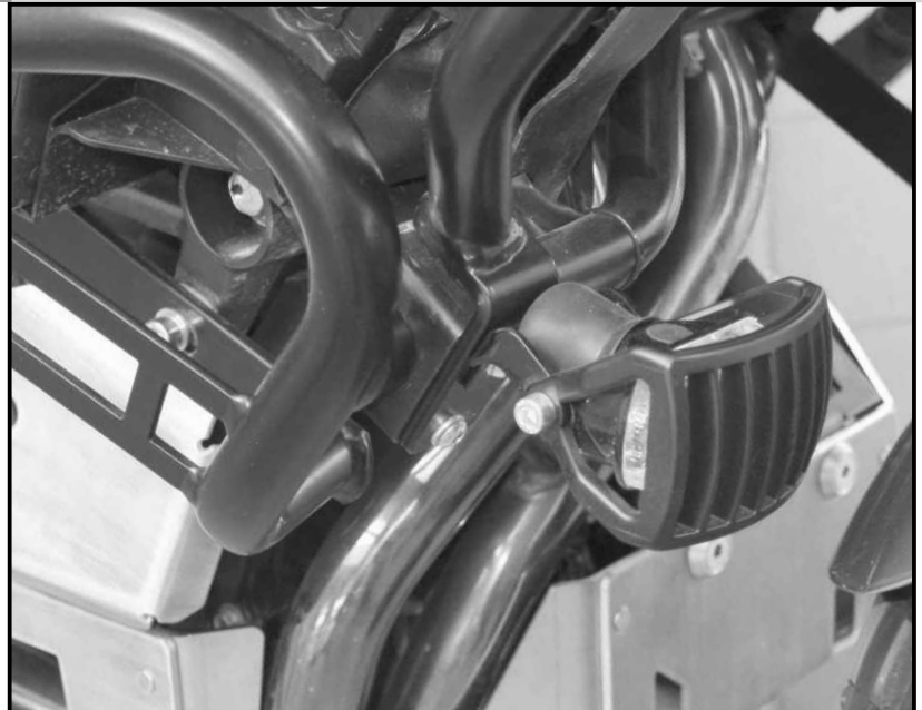
Picture shows optional protection grille for Microflooter 730.100
