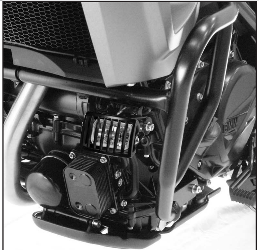
Picture shows optional protection grille for Microflooter 730.100
