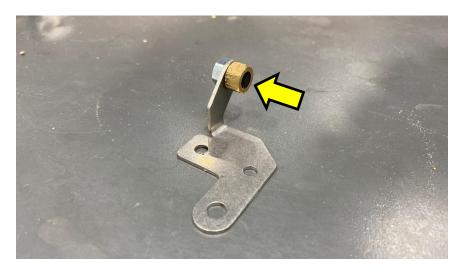
(3mm ALLEN) Bolt the sensor to the bracket as shown below. Blue Loctite is welcome here.
