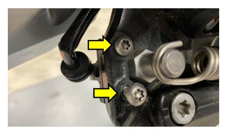
(10mm SOCKET or WRENCH) Remove the magnet from the kickstand.
