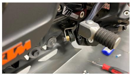
If you have an Arrow Decat system, the sensor can be mounted up further using the left side sump bolt.
