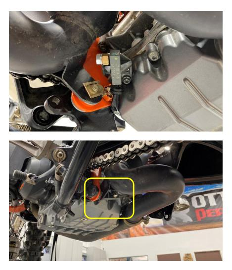
Alternatively, you can use the extra tab provided to move the sensors up somewhere much safer so that no damage can leave you stranded but this will take quite a bit more disassembly as the wire is behind quite a few items.
