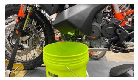
(GLOVES / SAFETY GLASSES / PLIERS) Using pliers, gently twist the Oetker clamp back and forth until the band comes loose enough to be removed from the stock plastic spigot.
