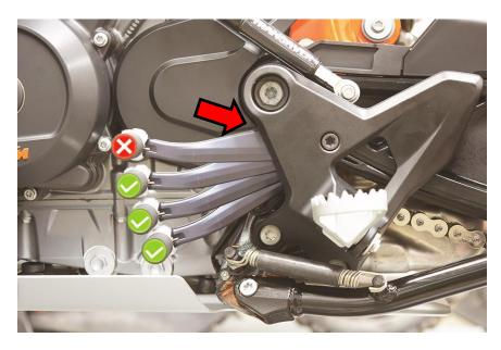
6. If a Vanasche sprocket cover is used, it will work with this part without issue and will not contact anything.
