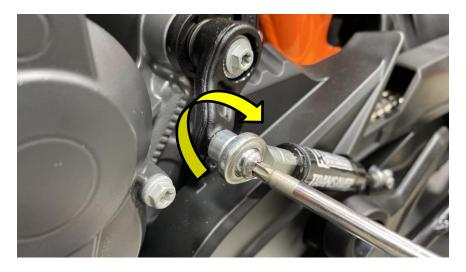
4. (T30 TORX) The TRANSAVER itself is not adjustable on the Adventure model due to the shortness of the linkage. Due to this adjustment to the height of the shift pedal will need to be performed at the upper lever similar to a dirt bike by removing the lever and moving to the next spline.
