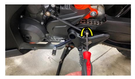
2. (T30 TORX) Locate the shorter of the two supplied button head TORX bolts and attach the Transaver as shown below. The sticker covers bare metal so do not remove it or the body may corrode, and the part will not look as cool.
