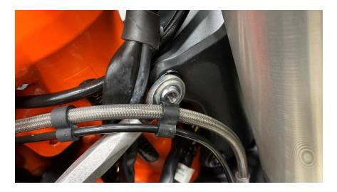
Very lightly snug the top bolts, then lightly snug the bottom two, then go back and tighten the top bolt and the remaining two. The holes are slotted to allow for possible differences between different frames and if you tighten one before the other there may be gaps under the part.
