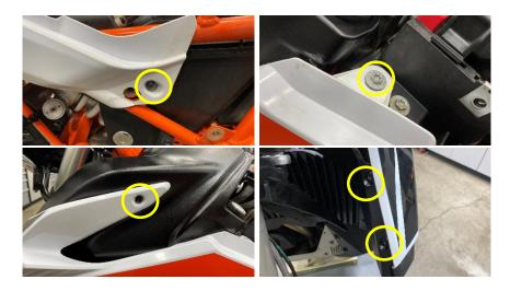
(6mm HEX) Remove the 4 fuel tank screws.
