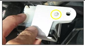
4. Replace the OE Screw removed in step 2 while holding the Reservoir Protector in place.
