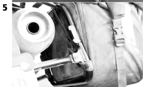
**EN** Now route both ROKstraps underneath and behind the pannier frame, loop them around the top rod and close the buckle. Tighten the straps until the bags are firmly fitted.
