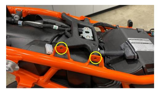
(T30 TORX) Remove the LEFT side fender well bolt.
