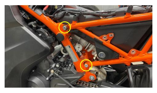
At this point, the left subframe can be removed. Start pushing out at the back LEFT corner and twist out.
