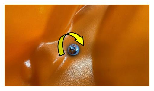
Reinstall the drain boots in the splash guard.
