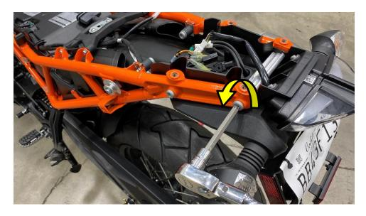
(T45 TORX) Remove the two 8mm left passenger peg bolts.
