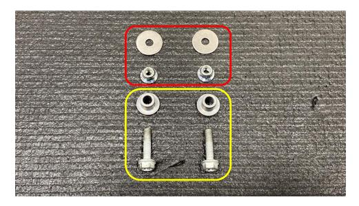
(PRO EDITION) Insert the spacer hats and bolts indicated above that originally were removed from the bottom of the stock airbox from this same location up through the BOTTOM of the rubber grommets in the subframe.
