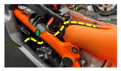
Push the fuel line connection back onto the spigot until you hear an audible click, then push up on the green locking tab. Pull out to make sure the spigot is properly locked on.
