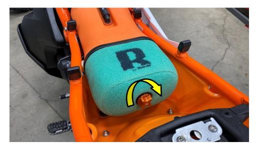
Make sure the base of the filter is evenly seated completely around the flange of the filter plate. You can feel this across the bottom where you cannot see. Once this has been ensured, you may tighten the bolt with a mild torque with your fingers.
