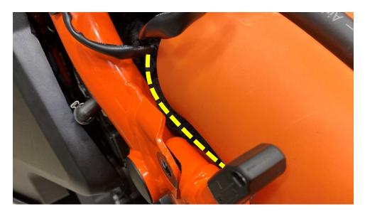
Route the harness above the rubber bumper. NOTE: You may keep these bumpers on the subframe. They will now keep the Rottweiler Intake airbox centered and will not come off.
