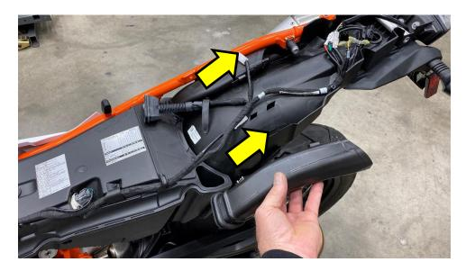
(CUTTERS) Cut the 4 zip ties indicated below. 2 on the airbox and harness, 1 on the crankcase breather and 1 at the harness at the rear.
