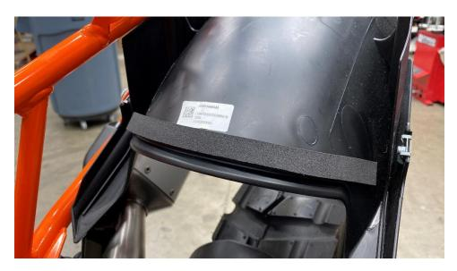
Work the splash guard into the position shown below, lining up the four holes to the filter plate. The splash guard will need a little coaxing under the upper right frame rail.
