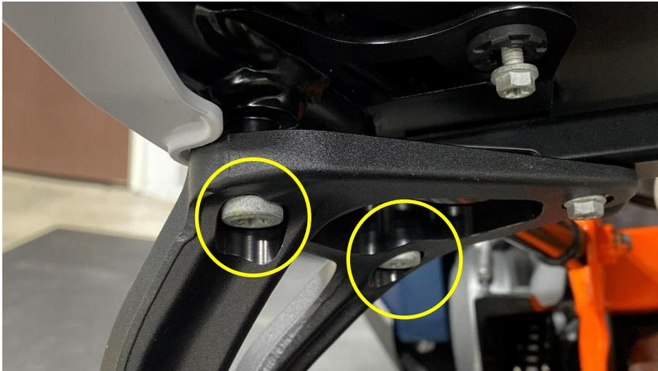
(T45 TORX) Remove the two front subframe bolts.
