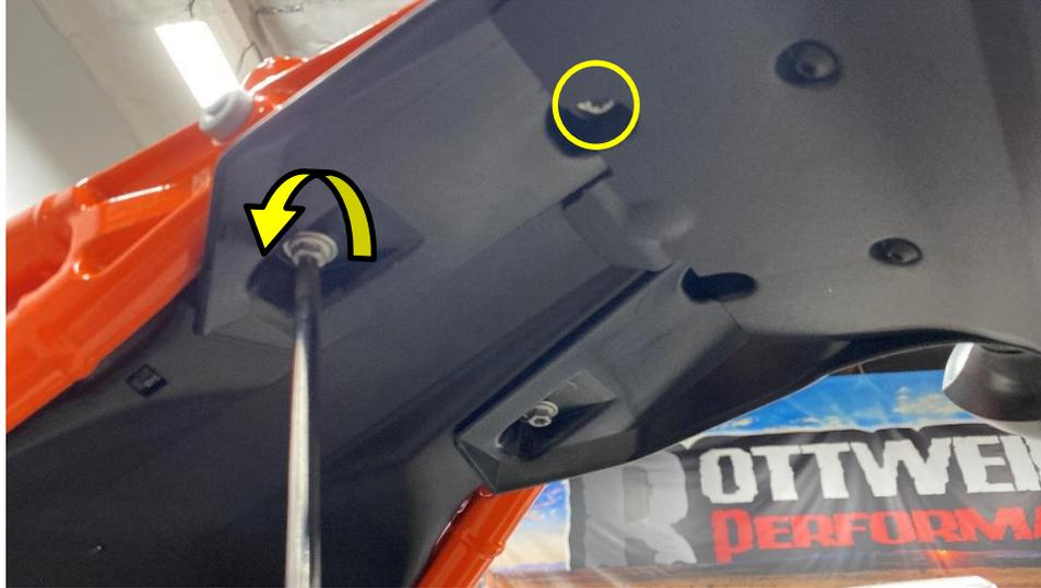
(T30 TORX) Remove the left passenger peg 6mm bolt and the two left subframe bracing bolts through the hole in the passenger peg.
