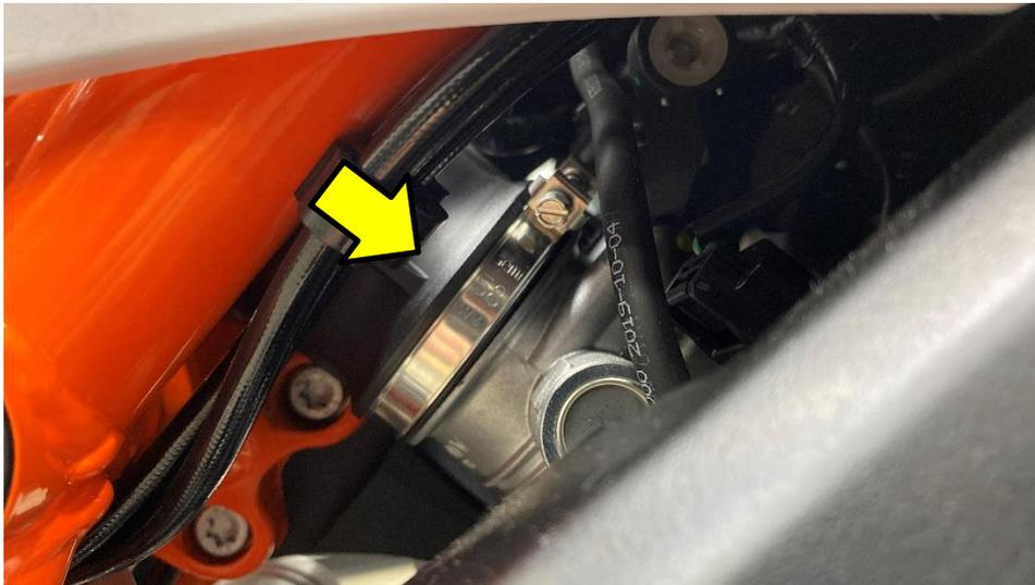
(6MM SOCKET + EXTENSION) Tighten the hose clamps on both sides.
