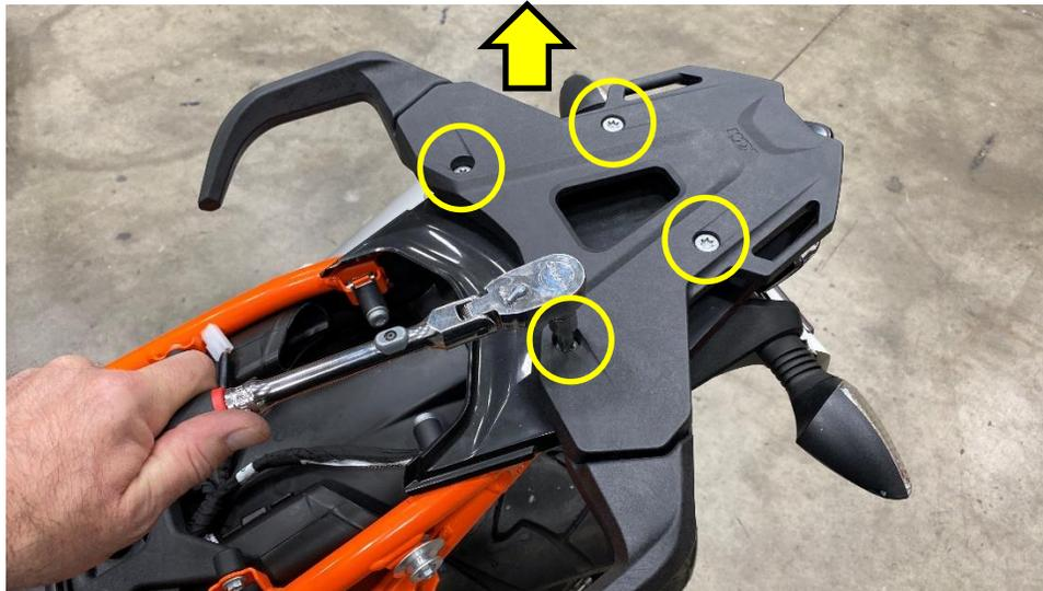
(T30 TORX) Remove the two RIGHT hand seat latch mount bolts.
