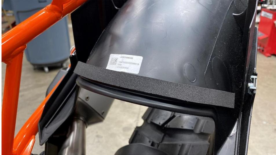
Work the splash guard into the position shown below, lining up the four holes to the filter plate. The splash guard will need a little coaxing under the upper right frame rail.
