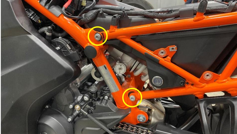
At this point, the left subframe can be removed. Start pushing out at the back LEFT corner and twist out.
