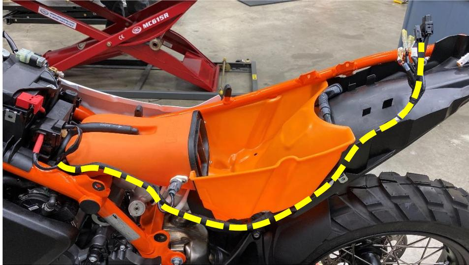
Cut the zip tie holding the seat latch cable shown below to free it to be repositioned. This is because you will now route the cable in a better way.
