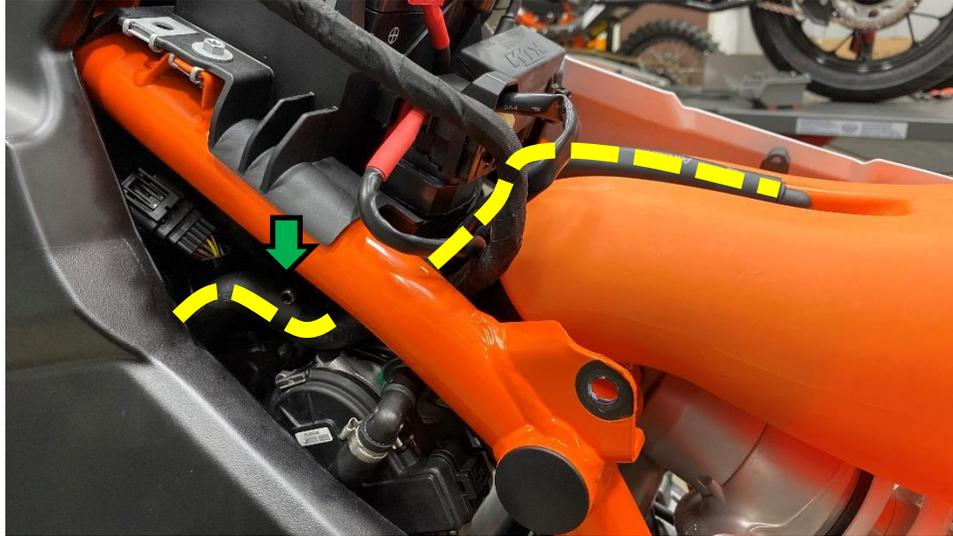
Push the fuel line connection back onto the spigot until you hear an audible click, then push up on the green locking tab. Pull out to make sure the spigot is properly locked on.
