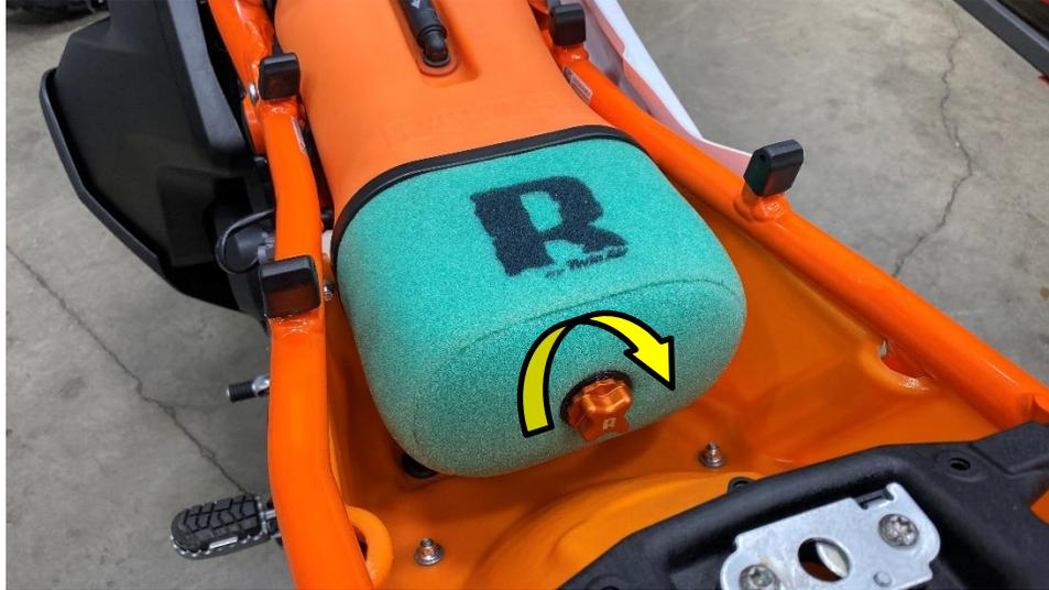
Make sure the base of the filter is evenly seated completely around the flange of the filter plate. You can feel this across the bottom where you cannot see. Once this has been ensured, you may tighten the bolt with a mild torque with your fingers.
