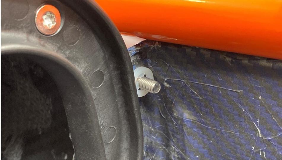
(3MM ALLEN + 8MM SOCKET) Thread on the nylon locking 5mm flange nuts and lightly tighten them. They do not need to be overtightened.
