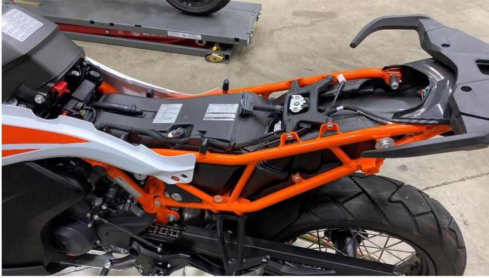
(T30 TORX) Remove the battery cover. This is only to access the left fairing bolt.
