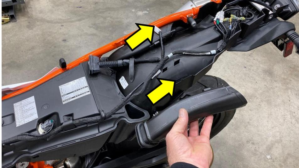
(CUTTERS) Cut the 4 zip ties indicated below. 2 on the airbox and harness, 1 on the crankcase breather and 1 at the harness at the rear.
