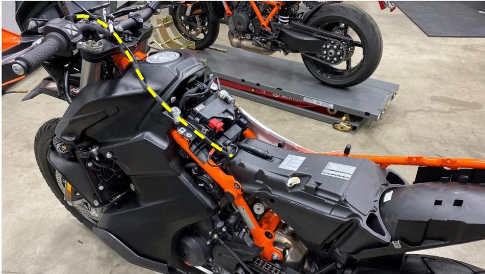
(T20 TORX) Remove the temperature sensor. You will reuse the temp sensor but not the screws.
