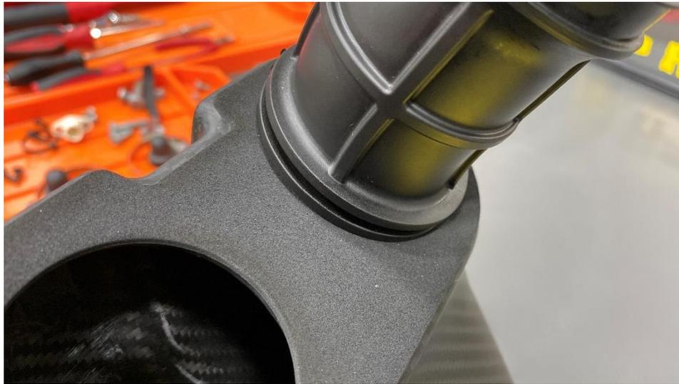
Using a blunt tool, start working the rubber stack's first flange into the hole by pushing it inward, taking care not to damage the foam layer. Once over half the flange is into the hole, it will start to pull itself in and help you along.
