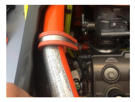
5. Locate the smaller cushion loop clamp and install it as shown below.
