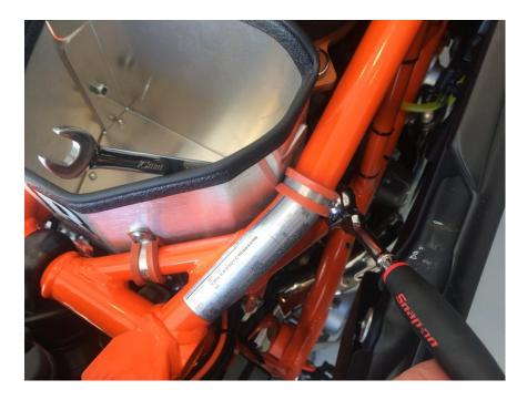
16. Ensure that the bottom of the Dog House is not touching the valve cover or any electrical components or wires.
