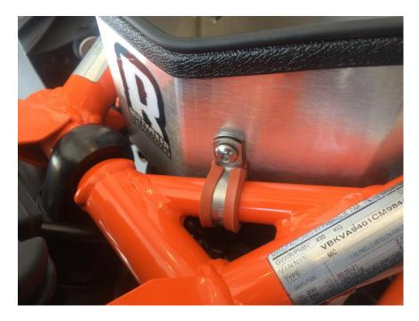
13. Now tighten only the bolt in the smaller cushion loop clamp.
