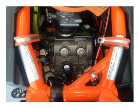
7. Drop the Dog House down into the frame and behind the Rottweiler Intake Filter. Be careful not to pull any of the rubber protectors off of the stainless bands as the Dog House may rub on them when you drop it into the frame. Some glass cleaner can help lubricate them and will simply evaporate after the install.
