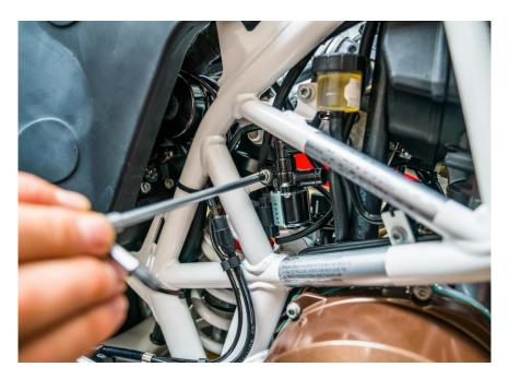
10. Locate the blue colored dongle (pictured in black below) and insert each pin into the harness plug that was plugged into the SAS valve. NOTE: There is no plug in existence for this connection so this is the method we chose to insert the dongle.
