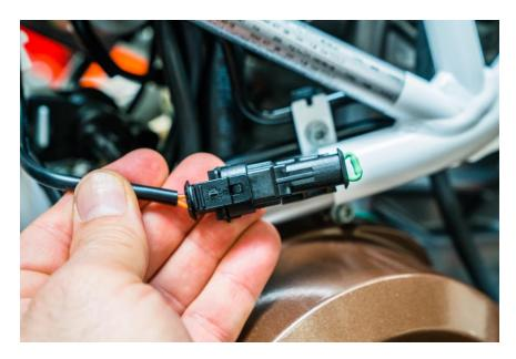
22. Zip tie the two dongles to the frame in a safe place.
