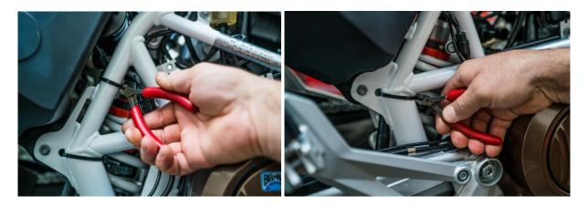
18. Remove the 'Y' section of the hose and rejoin the fuel tank hose to the other hose on the 'Y' adapter of the same diameter with the straight barbed fitting.
