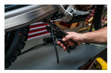
20. Remove the canister valve from the tab on the frame and unplug the electrical connection.
