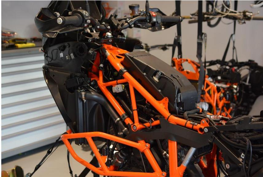
2. Remove the plug on the temperature sensor.
