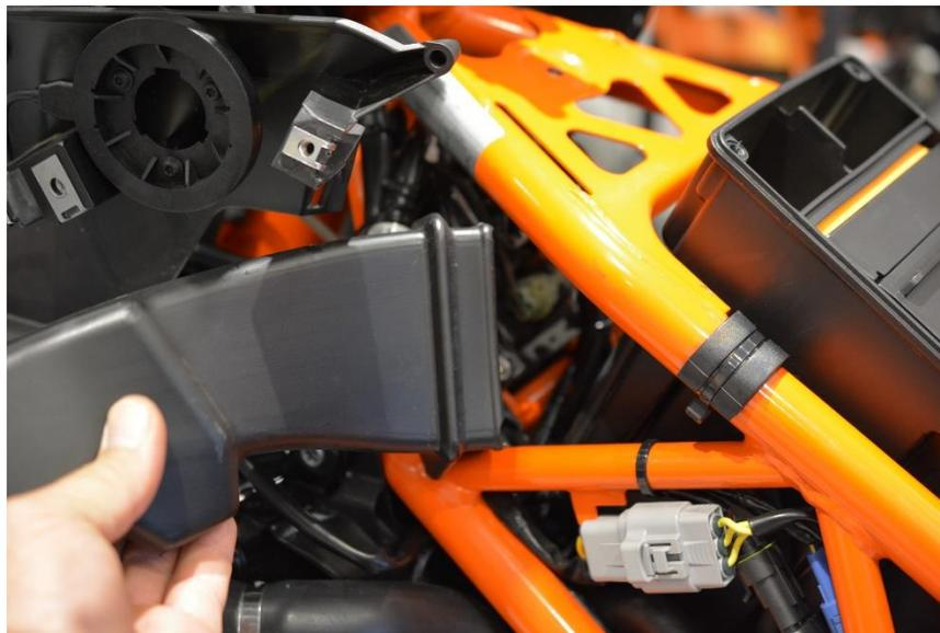
7. T30 or 8mm – Remove the front cylinder SAS cover.
