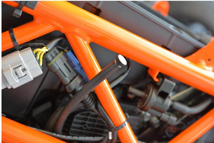
29. Disconnect the plug and plug in the supplied canister dongle.
