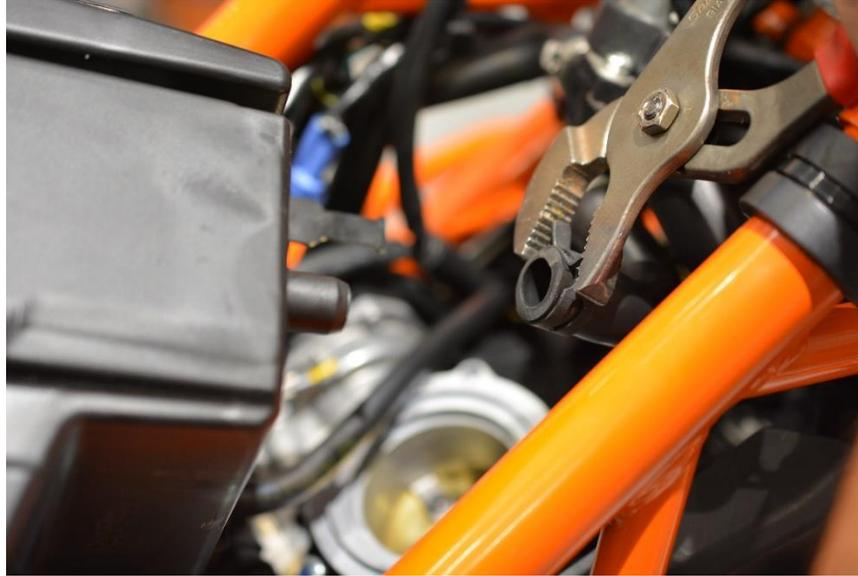
12. There is one more plugged drain hose attached to the bottom of the airbox. Trace it down, remove any rubber straps and now pull out the bottom portion of the stock airbox.
