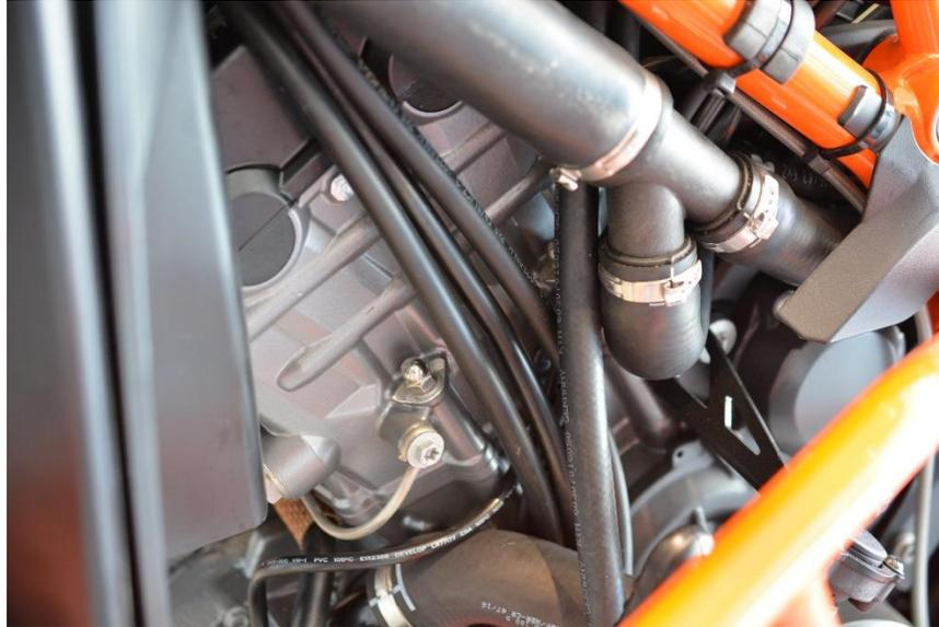
27. Locate the canister valve on the left side of the upper frame and disconnect the front hose. This leads to a 'Y' connector that splits and goes to the throttle bodies and draws a slight vacuum.
