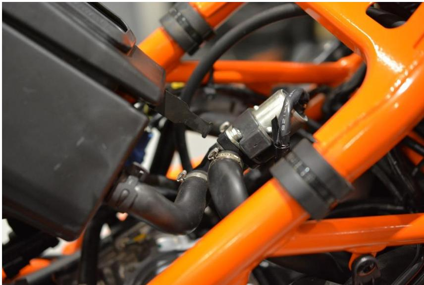
11. Remove the hose from the bottom of the airbox.
