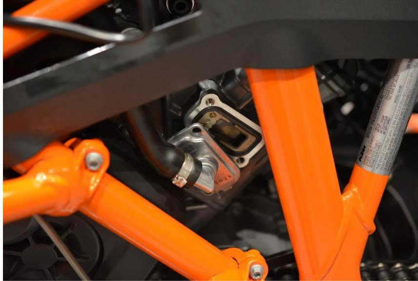
14. Unplug the SAS valve's electrical connection. You will pull up on this particular connection's locking tab.
