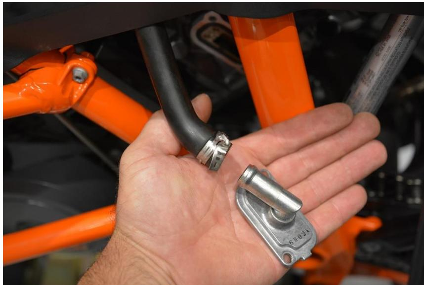
16. Extract the SAS system completely by bringing it up through the frame. You should end up extracting the parts below.
