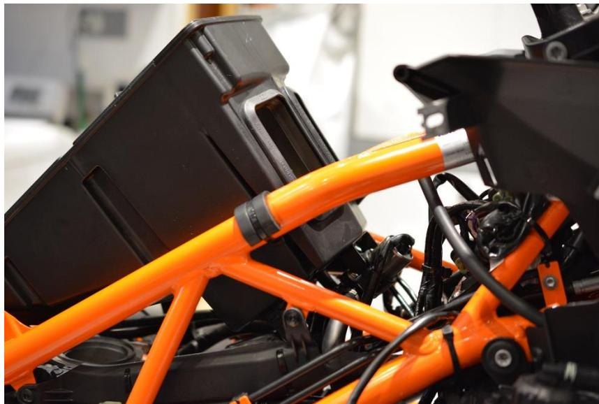
9. Push the SAS valve off of its rubber stakes and off of the bottom of the airbox.
