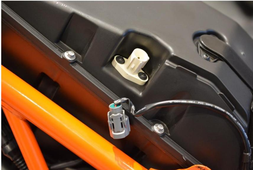
3. 6mm socket x 8 - Remove all 8 screws on the air box lid.
