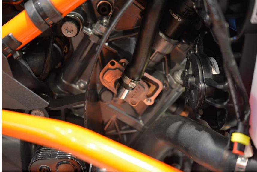
8. Pull the airbox back and up and locate the SAS valve attached to the bottom of it.
