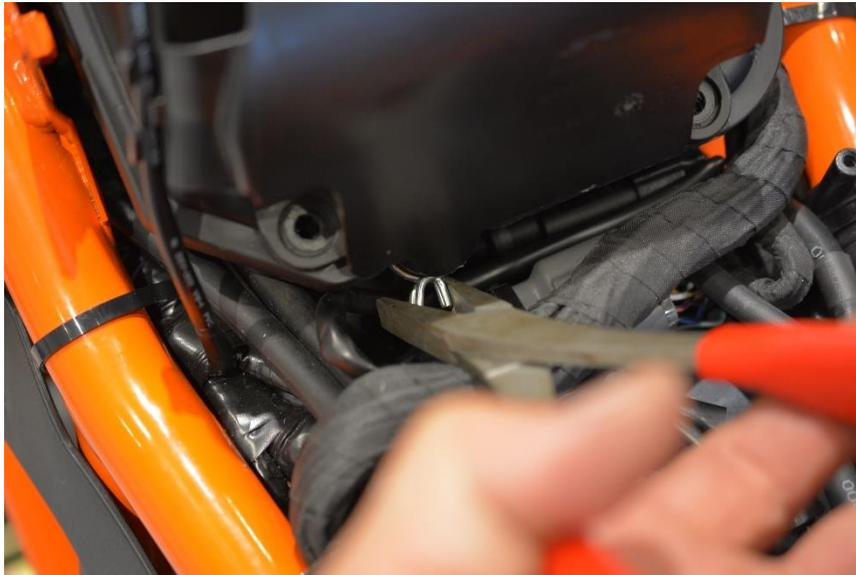
5. T30 x 2 - Remove the velocity stacks.
