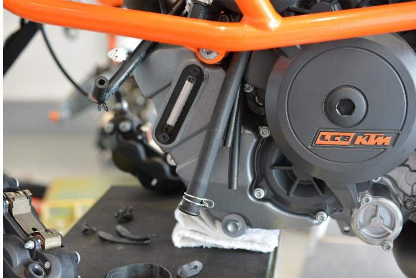
24. Trace it up and locate the 'Y' connector and disconnect it.
