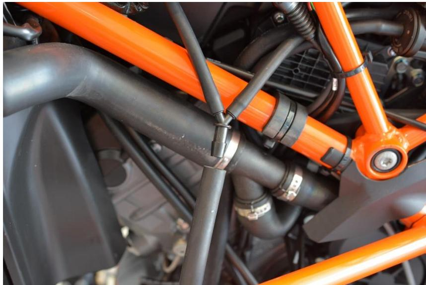
25. Extract the 'Y' connector and the two hoses attached to it.
