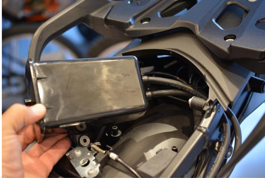
22. Locate the two hoses shown below and pull them through from the back to the middle of the bike just behind the airbox.
