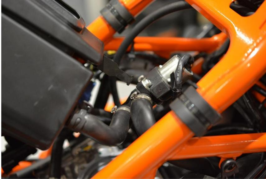
10. Through the side of the frame, locate the short line that connects the SAS valve to the bottom of the airbox and compress the spring clip holding it.
