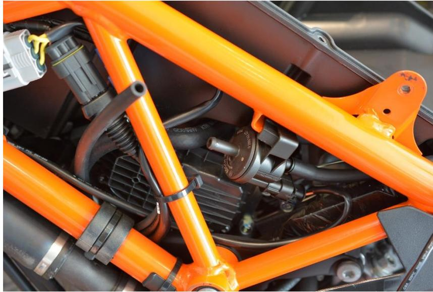
28. Plug the front line with the 8mm thumb screw. Tie it to the frame with a zip tie. You may also shorten this hose if desired before plugging it.
