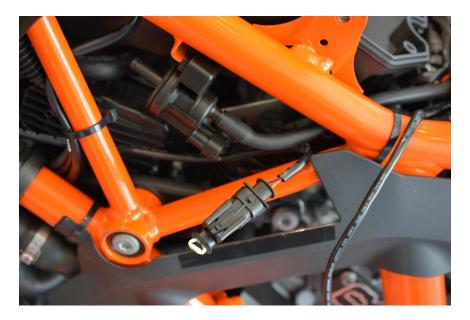
30. Remove the canister valve from the frame and extract it and the rearward hose.
