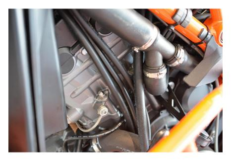
27. Locate the canister valve on the left side of the upper frame and disconnect the front hose. This leads to a 'Y' connecter that splits and goes to the throttle bodies and draws a slight vacuum.
