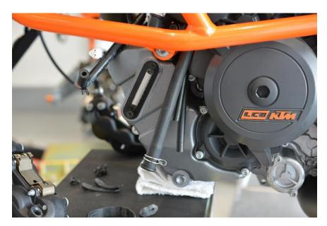
24. Trace it up and locate the 'Y' connector and disconnect it.
