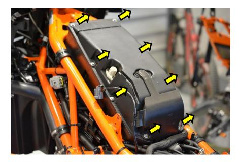
4. Pliers - Compress the crankcase breather line spring and remove the airbox lid.
